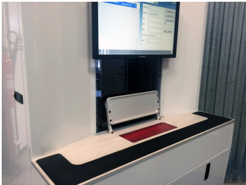
Photo above: The optional servo-controlled shutters (red) , prevent the user from accidentally inserting or withdrawing item from wrong compartment.
